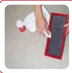
Place the filter on a flat surface and allow the oil to absorb for about 30 minutes. Clean any excess oil from the rubber and check that the filtering element has an even red colour. (Picture 7). If not, it is necessary to repeat the oiling process following the above instructions after which your filter will be ready for reuse.
