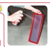
If using the aerosol spray version (Picture 6), hold the spray 15cm from the filter and spray the entire filter surface. Repeat the operation on the reverse side.
