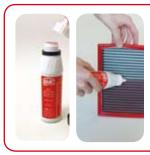
Remove the original top from the oil bottle. Make a small hole in the dispenser spout and screw it on the bottle (Picture 5A) For correct oiling we recommend passing over every filter pleat twice with the oil, repeating the operation on the reverse side. (Picture 5B)
