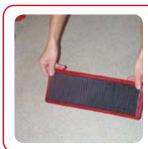
Remove larger dirt by gently tapping your filter on a flat surface (Picture 1). DO NOT use compressed air which may damage the filtering element.
