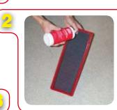
Apply the detergent evenly over the filter folds and allow to absorb for 10 minutes (Picture 2) DO NOT use caustic products such as petrol or oil. USE ONLY BMC DETERGENT.
