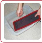
Wash your filter in cold water. Rinse well ensuring that dirt does not enter the filter pleats. (Picture 3) DO NOT use high-pressure water.
